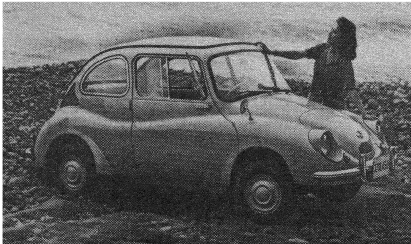
For export markets the Subaru 450 has a larger 423 c.c. engine developing 23 b.h.p. at 5,000 r.p.m. deep cowl head-lamps and heavier bumpers
