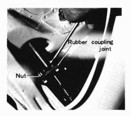
(c) Remove the (8 x 20 mm) bolts fixing the rubber coupling joint. Remove the steering shaft assembly installation bolt on the dashboard and slide the shaft assembly inward into the cabin. The joint and shaft will separate.
