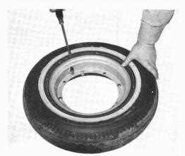
Remove the tube and lay the wheel on the floor. Insert a tire lever or a large screw driver between the tire and the rim. Bear down on the lever and separate the rim from the tire. Repeat this operation around the rim and one rim-half can be easily removed.
