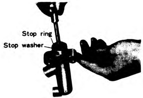
Fig. 5-36 Reinstalling stop ring
