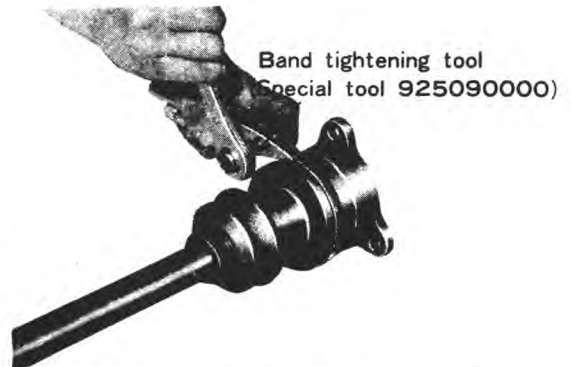
Fig. 4-48 Installing boot bands
