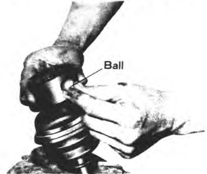
Fig. 4-41 Inserting inner race and C-type snap ring
