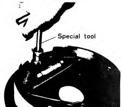
Fig. 5-9 Removing spring cable
