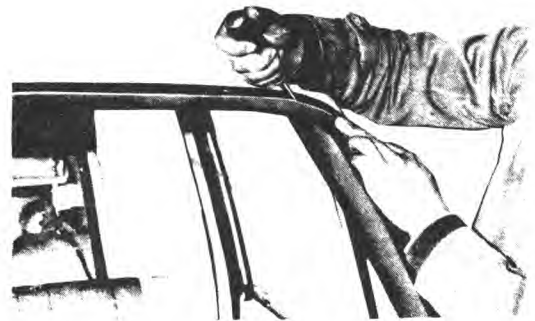
Fig. 13-69 Installing metal moulding
