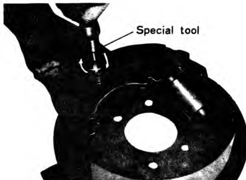
Fig. 5-10 Removing the shoe set spring
