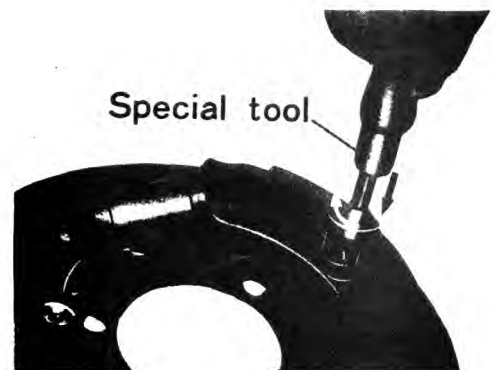
Fig. 5-25 Removing shoe set spring
